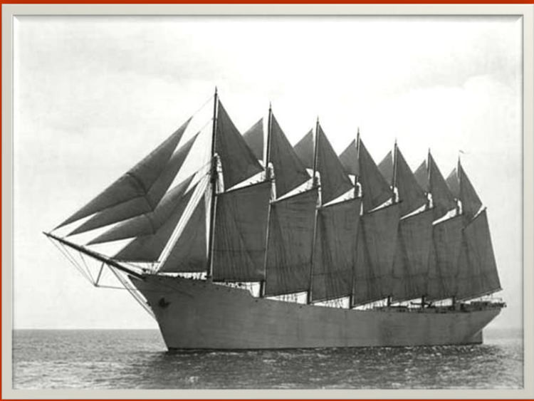
Constructed in 1902: 25 sails with 4,000 m 2 of total sail area
